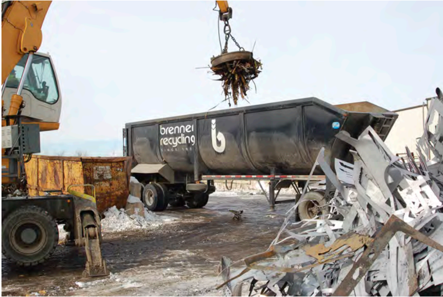
Brenner Recycling equips its three material handlers—two Liebhers and one Link-Belt—with a shear attachment, grapple, and magnet, giving it flexibility to move and process ferrous scrap in the yard. Above, a handler loads No. 1 steel into one of the company's newer dump trailers.
