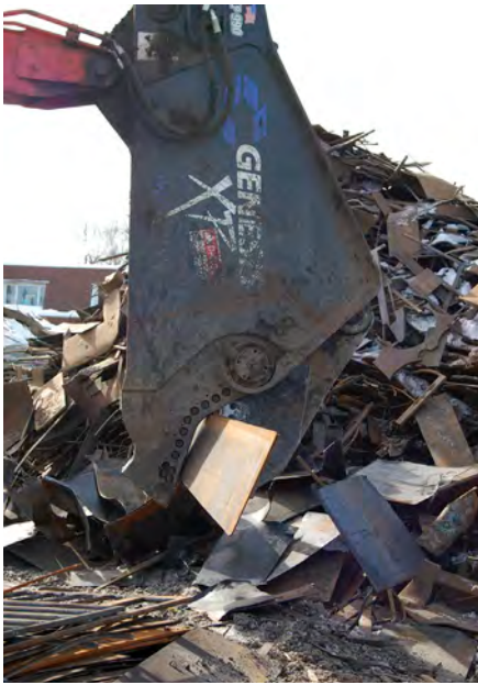
Brenner Recycling uses a Genesis shear attachment (left) to process plate and structural scrap into 3-foot and 5-foot lengths. The company also torchcuts (center) plate steel and other material that's too thick or unwieldy for its mobile shear. Its other main piece of processing equipment is a Mosley Gorilla baler (right), which handles nonferrous and paper scrap.
